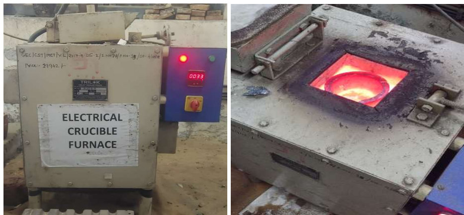
Figure 6-2 Electric Resistance Furnace at Dr. S & S. S. Ghandhy College of Engineering & Technology, Surat.
