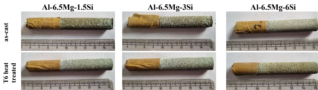
Figure 6-13 Surface morphology of Al-6.5Mg-xSi sacrificial anode specimens ( x = 1.5, 3, 6 ) after Anode performance measurement in both as-cast and T6 heat treated conditions.
